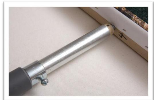
8. Bring the sleeves on the other side up to the tube one at a time and pull the rod and tube apart to stretch the canvas, then while holding them with one hand, tighten the screw with the other, or better have a helper stretch the canvas while you tighten.
