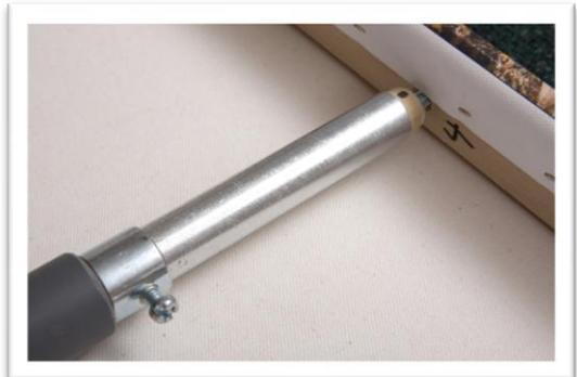
8. Bring the sleeves on the other side up to the tube one at a time and pull the rod and tube apart to stretch the canvas, then while holding them with one hand, tighten the screw with the other, or better have a helper stretch the canvas while you tighten.
